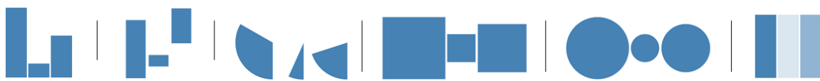
Figure 5-5. Difficulty in comparison increases roughly from left to right: comparing length with a shared baseline and with different baselines, comparing angles, comparing square areas or circular areas, and comparing color. Each of these shows three values in the proportion 5:1:3.
