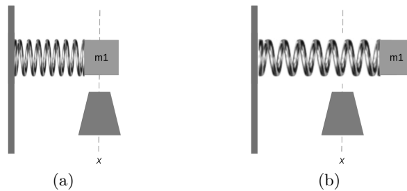
Figure 15.9: (a) When the mass is over the magnet it experiences a force in the direction of its motion. (b) When the mass is away from the magnet, no external force is applied.
