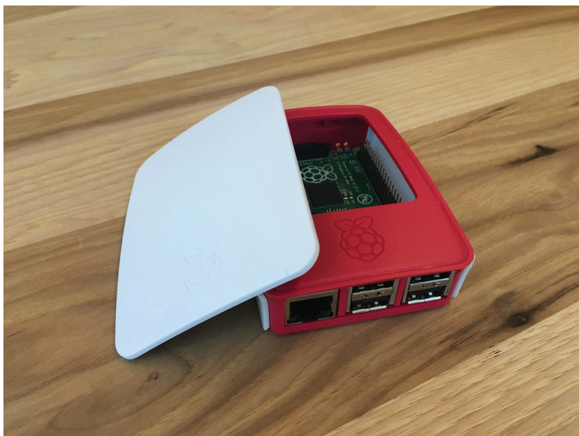
Figure1-7. With the official Raspberry Pi case, you can remove the top and sides to access the different parts of the board.
