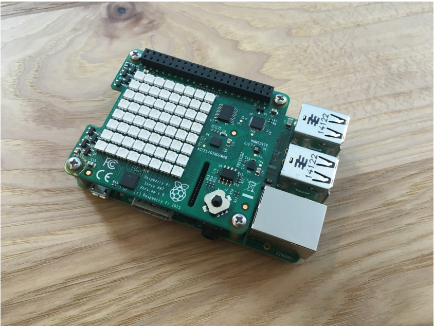
Figure 1-5. The Sense HAT add-on board includes an LED matrix, a suite of sensors, and a joystick input. It was designed for the Raspberry Pis that were sent to the International Space Station.
