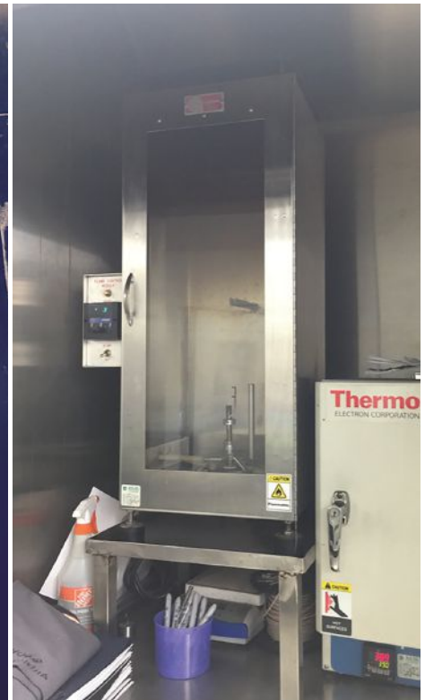
Example of a vertical flame resistance test that determines if a textile will continue to burn after ignition is removed. Afterflame, afterglow, and char length can be measured.
