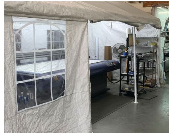
No, a printer in a tent is not a climate-controlled condition. Fluctuations in humidity and temperature throughout the year affect color balance – an overlooked variable that directly affects product consistency.
