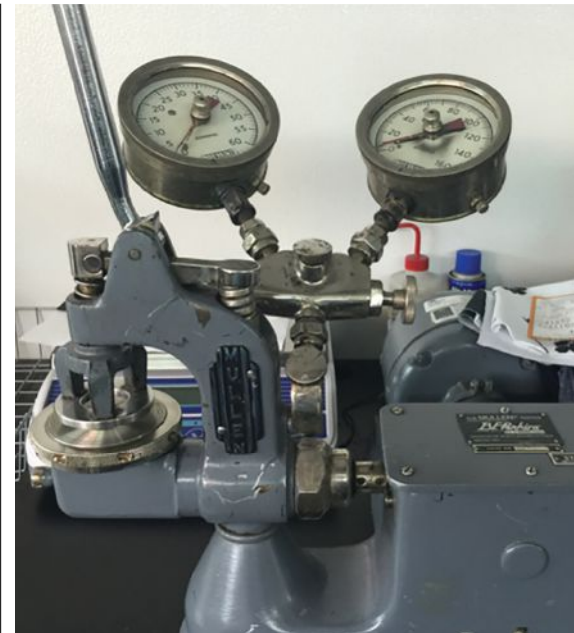
A burst strength test, commonly performed on textiles with stretch, measures how the fabric handles pressure.
