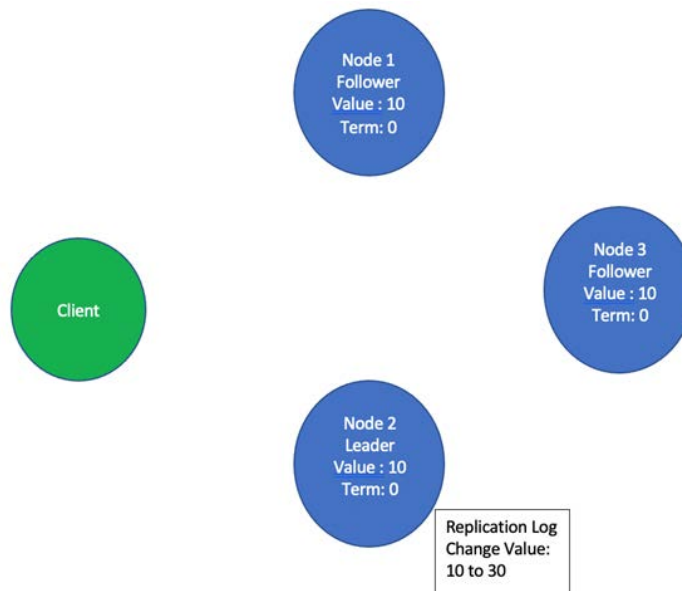
Figure 2.8 – Node 2 appends the entry to change the value from 10 to 30 in its replication log
