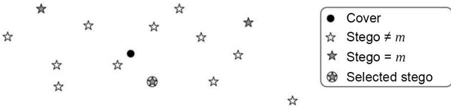
Figure 5.2. Coding for steganography: the coding system generates several code words associated with the same message, m , in order to select the one that is closest to the cover content, and so minimizes the distortion between the cover content, and the stego content
