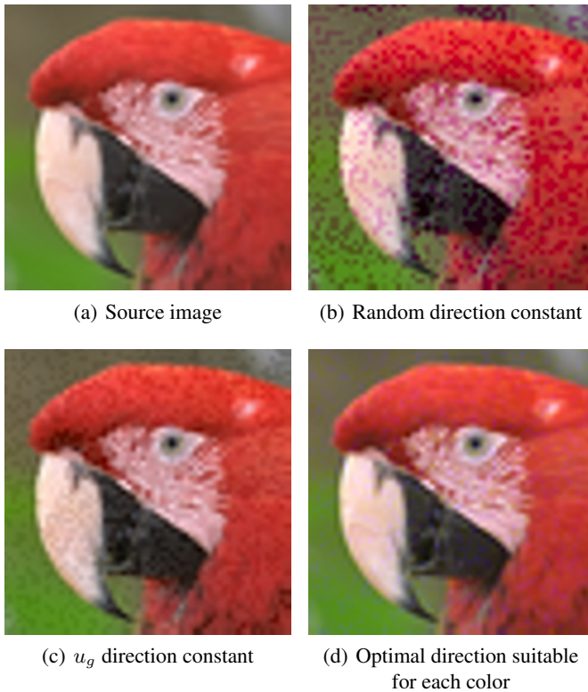
Figure 4.2. Example of inserting a mark with different approaches and direction vectors with equivalent digital distortion (overall, the signal to noise ratio is equivalent for the three images). The image used is a cropped version of the image kodim23.png from the Kodak Image Database (available at: http://r0k.us/graphics/kodak/kodim23.html )
