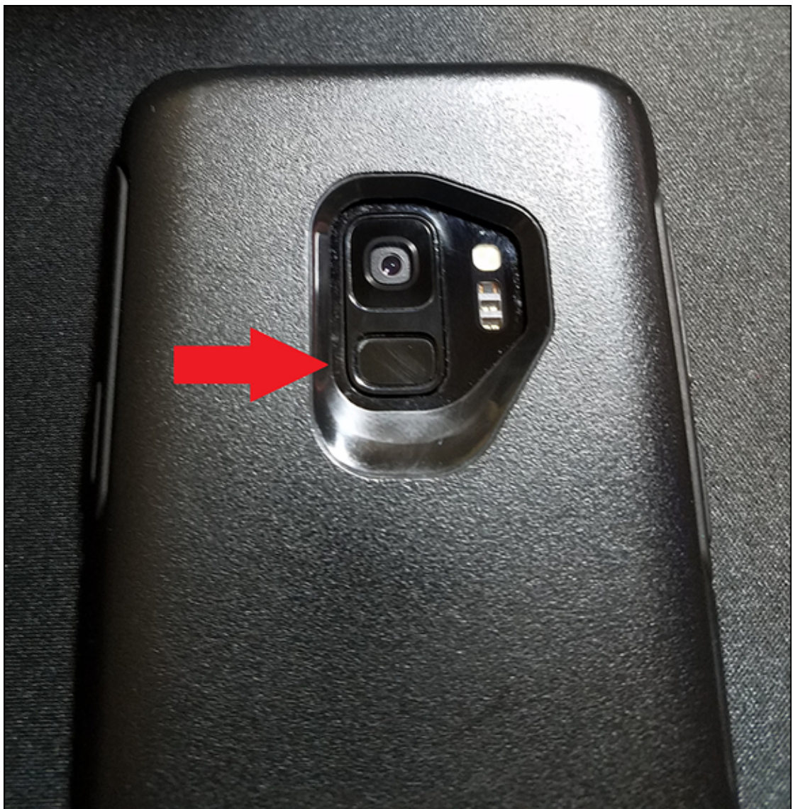
FIGURE 8-3: A phone fingerprint sensor on a Samsung Galaxy S9 in an Otterbox case. Some phones have the reader on the front, while others, like the S9, have it
