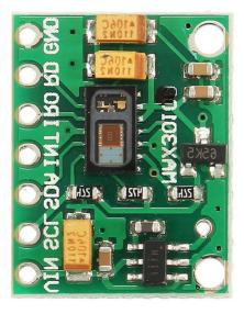
The MAX30102 operates on a single 1.8V power supply and a separate 5.0V power supply for the internal LEDs. Communication is through a standard I2C-compatible interface. The module can be shut down through software with zero standby current, allowing the power rails to remain powered at all times.
