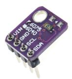
VEML6040 provides excellent temperature compensation capability for keeping the output stable under changing temperature. VEML6040's function are easily operated via the simple command format of I2C (SMBus compatible) interface protocol.
