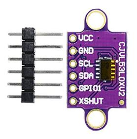
The VL53L0X's 940 nm VCSEL emitter (Vertical Cavity Surface-Emitting Laser), is totally invisible to the human eye, coupled with internal physical infrared filters, it enables longer ranging distances, higher immunity to ambient light, and better robustness to cover glass optical crosstalk.
