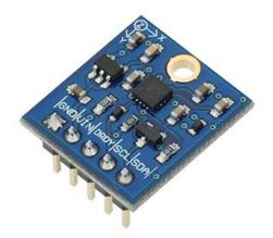
The HMC5883L utilizes Honeywell's Anisotropic Magnetoresistive (AMR) technology that provides advantages over other magnetic sensor technologies. These anisotropic, directional sensors feature precision in-axis sensitivity and linearity.
