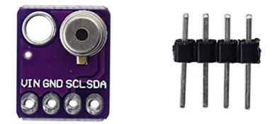
The infrared thermometer comes factory calibrated with a digital SMBus output giving full access to the measured temperature in the complete temperature range(s) with a resolution of 0.02 °C. The sensor achieves an accuracy of  $\pm 0.2$  °C within the relevant medical temperature range. The user can choose to configure the digital output to be PWM.
