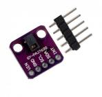
It also offers built-in proximity detection in sensing approaching or departing object from the sensor. The PAJ7620 is designed with great flexibility in power-saving mechanism, well suit for low power battery operated HMI devices.
