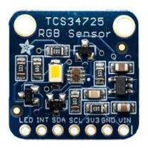
Features Integrated IR blocking filter 3.8M:1 dynamic range Four independent analog-to-digital converters A reference channel for color analysis (clear channel photodiode)
