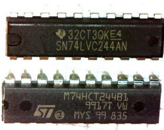
Figure 2-1. Two useful level interfacing chips
