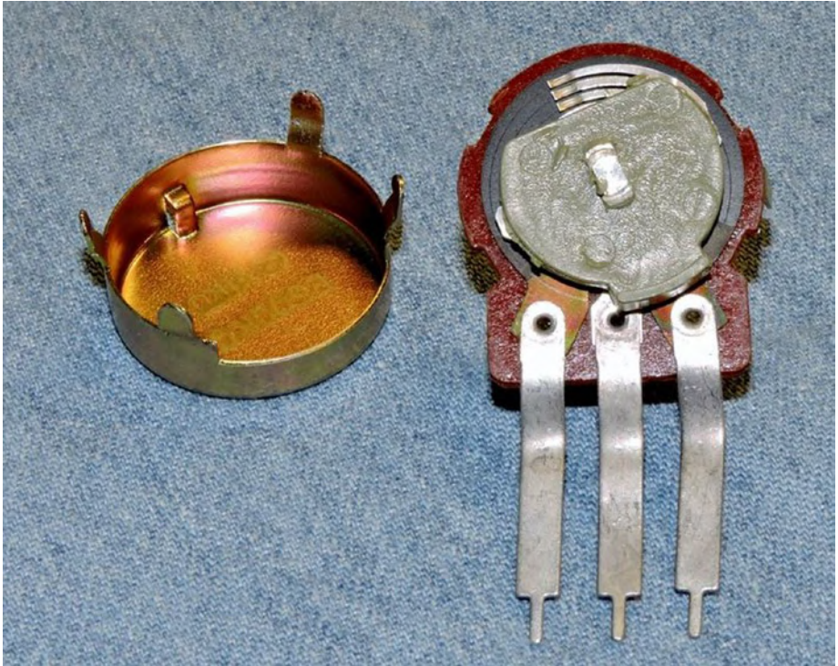
Figure 7-2. The revealed innards of a PCB potentiometer
