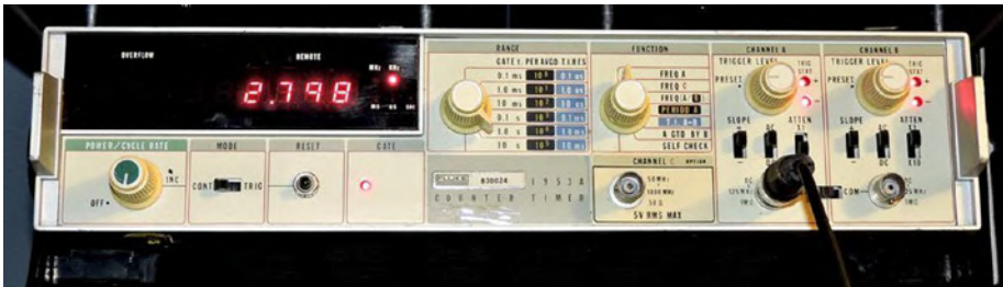
Figure 5-3. An old Fluke 1953A frequency counter used to determine the 3.3V formula for C_p by measuring frequency
