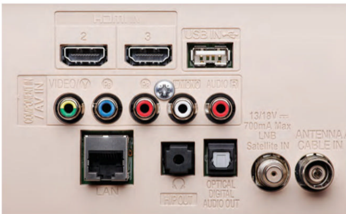
Back of TV showing two HDMI ports (top left).
