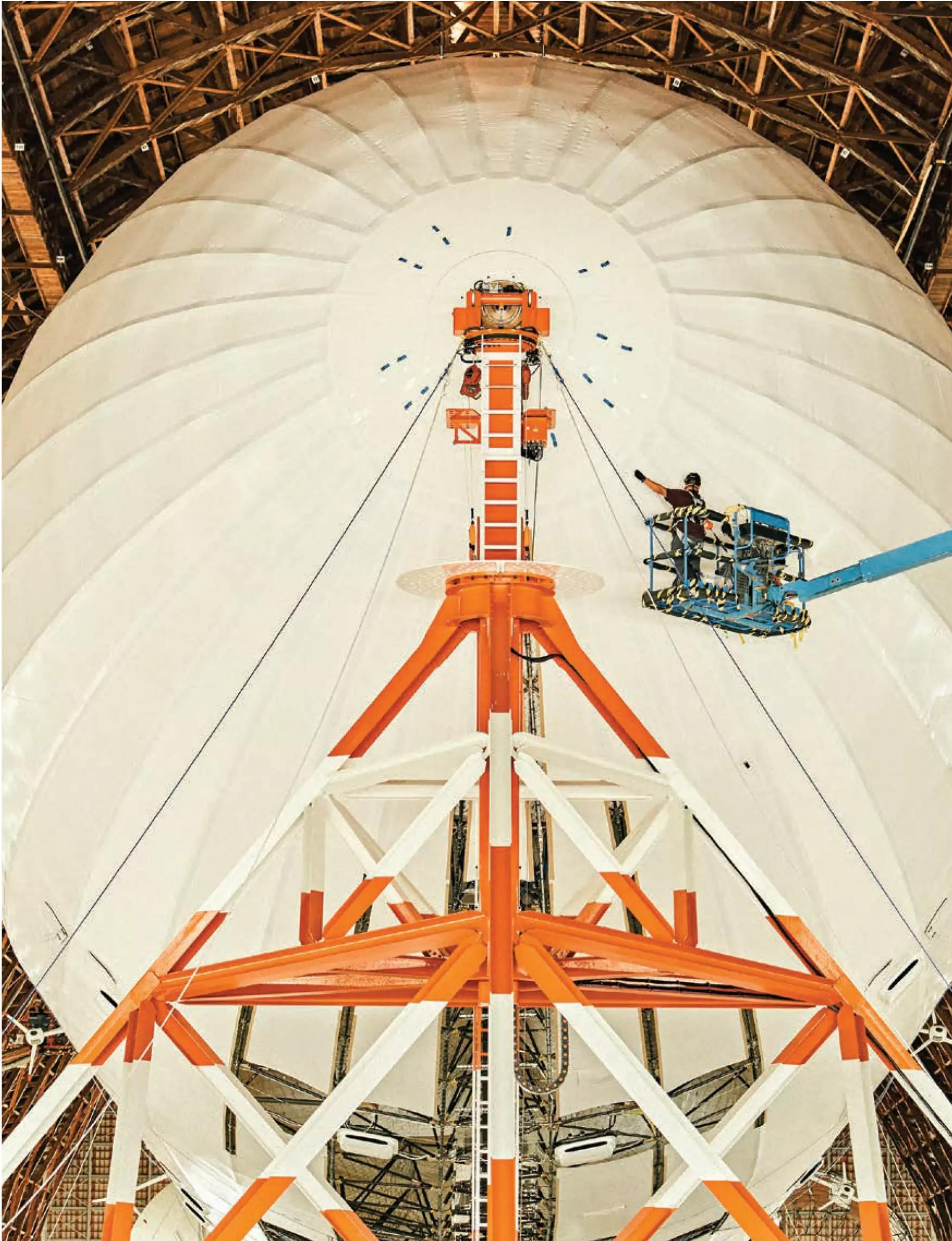
◀ Brin's airships, with carbon-fiber tubing, would be lighter and sturdier than the ones from a century ago
