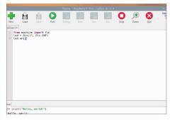
Type it into the upper section of Thonny, save it as LED.py (for example) and run the code. The LED will light up. But, let's explain what's going on here.
