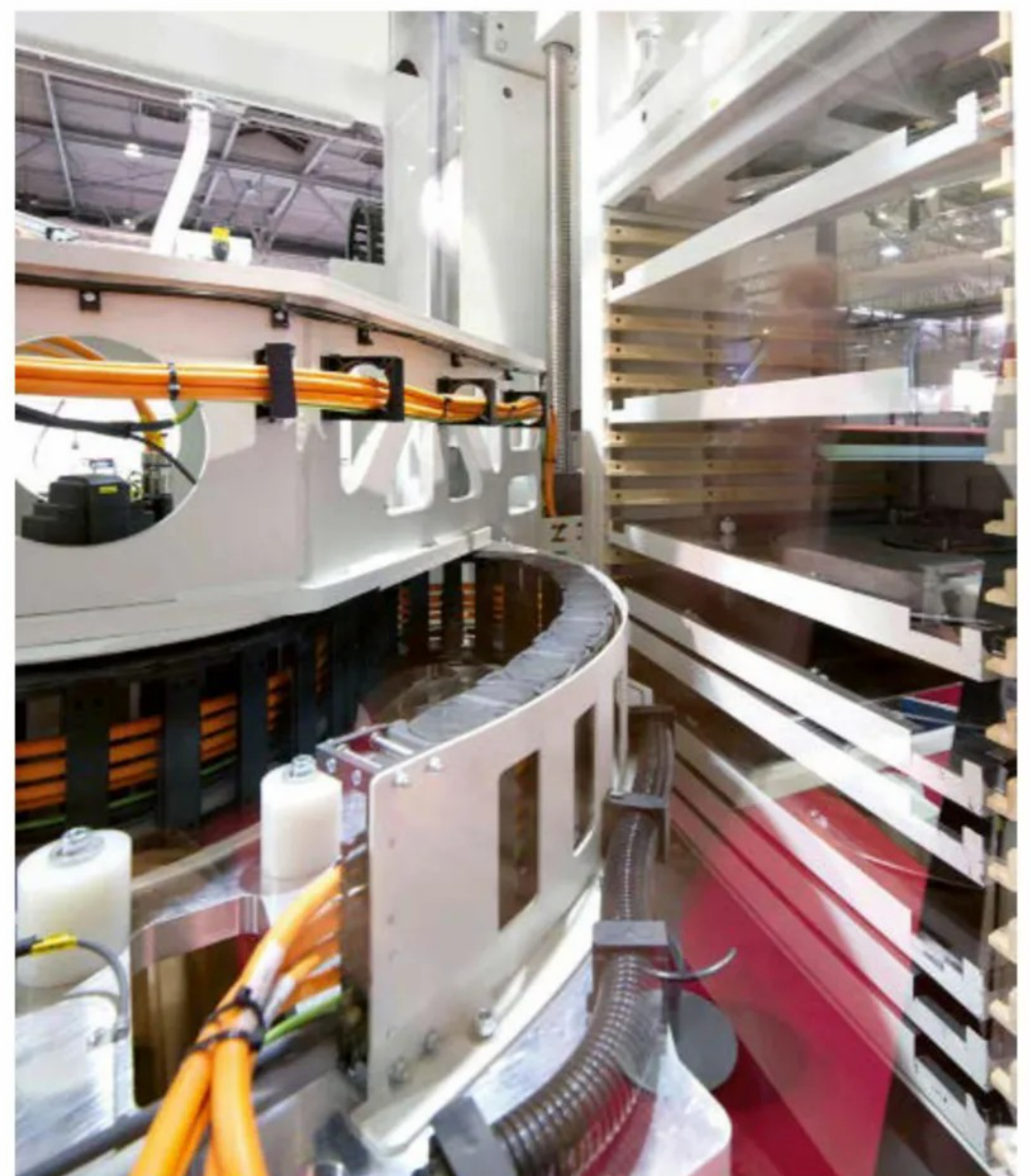
System for automatic needs-based supply and processing of material in the edge joining area
