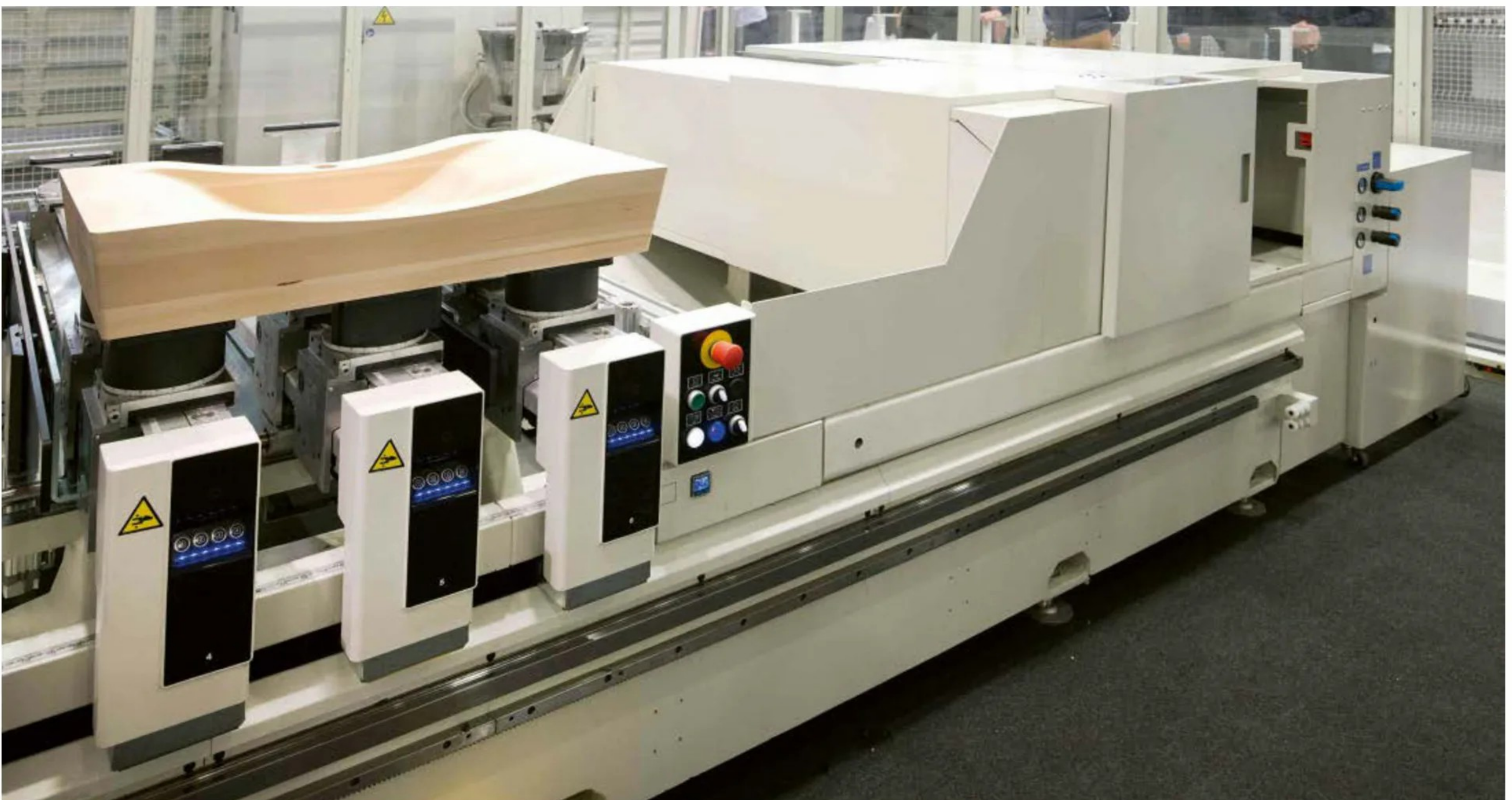
Up to 35 tools are stored in a new device called Caddy 35, close to the machining head.
