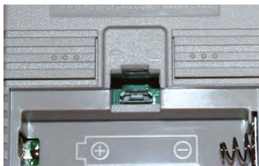
A micro USB port under the GPI's battery cover can provide USB peripheral connectivity via a powered hub, but reliability varies greatly from hub to hub
