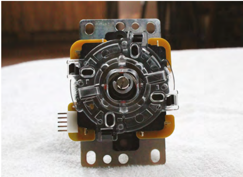
▲ The underside of a Sanwa JLF-TP-8YT joystick. Note the e-clip securing the central shaft
