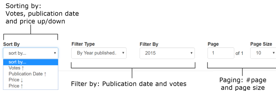
Figure 2.10 The three commands, sorting, filtering, and paging, as shown on the example book-selling site.
