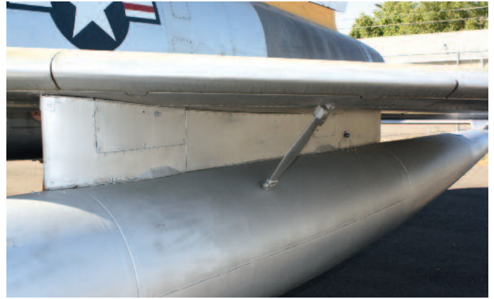
The attachment of the auxiliary tank under the wing has a streamlined body to reduce drag.
