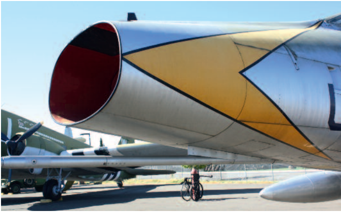
The air intake to supply the engine is designed as a thin lip on the F-100D to reduce air resistance. In addition, this special design of the inlet optimises the supply of air to the engine, which has led to an increase in the performance of the Pratt & Whitney J57 turbine.
