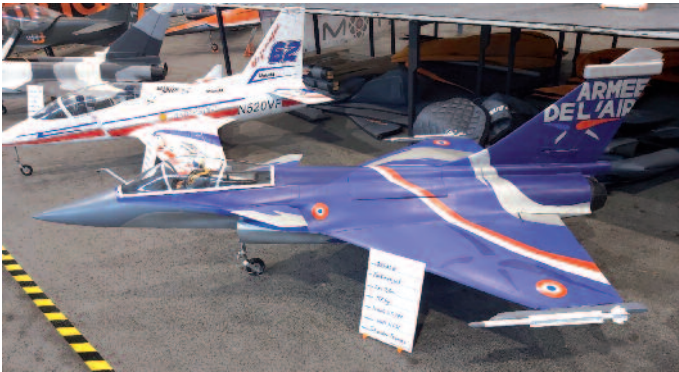
The Rafale model on display was very impressive and had a colourful special French Air Force livery. The wingspan is 1,600 mm and the take-off weight is 17,000 grams. The all-GFK Rafale belongs to Thomas Schaidler and is powered by a Frank ST-180.
