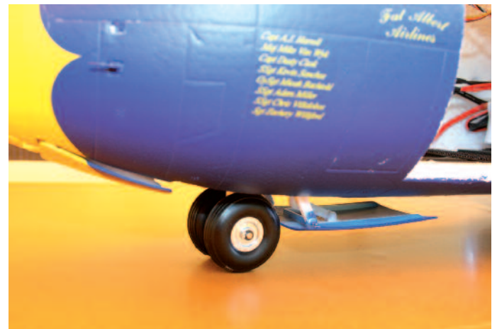
The plastic rims of the nose gear with twin tires could not withstand the stresses of rolling and had to be replaced with aluminum rims.
