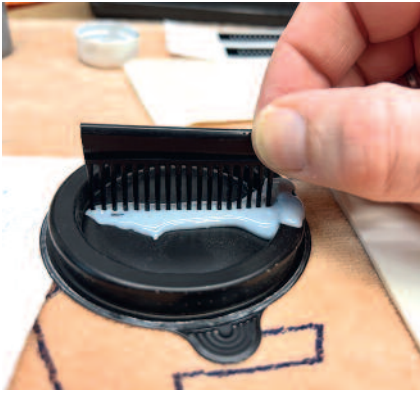
The combing method is basically simple: dip the rivet comb into the glue...
