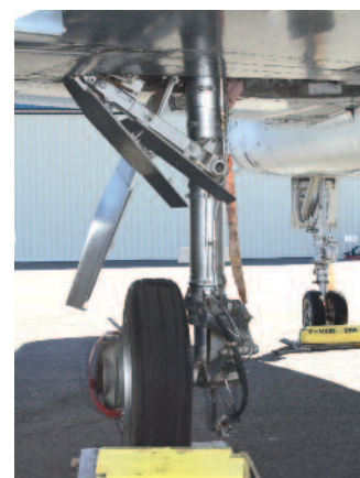
Like the nose gear, the main gear is hydraulically sprung against shocks during landing. However, the undercarriage leg has only one high-pressure wheel.
