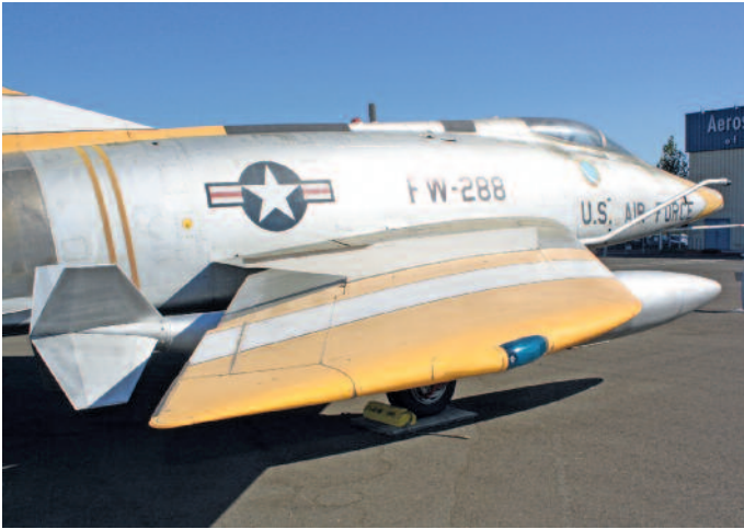
The wing of the F-100D has a sweep of 45° and a seven percent thickness ratio at the thickest point and a 3.5% ratio at the weakest point. Compared to the previous variants, the D-pattern has leading edge slats.
