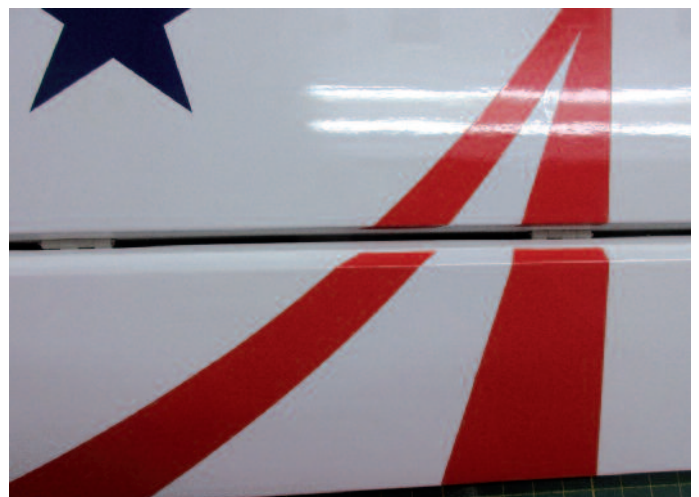
Without recessed hinges, the slits are too large.
