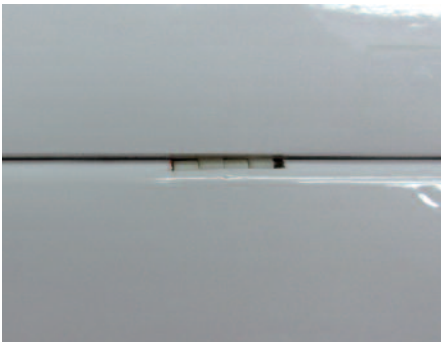
Attachment of the inverted control horns to the airbrake.
