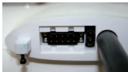
The controllers and motors as well as the servos for aileron and landing flaps are supplied with power via the fuselage and wing plug connections. No cable clutter, a perfect solution.
