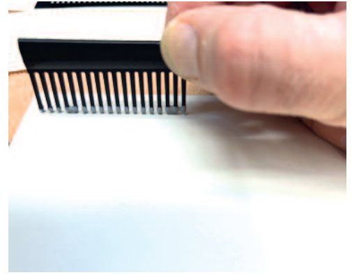
Then press the rivet comb into the desired place and pull it away upwards.
