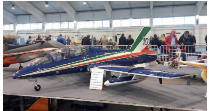
The Aermacchi MB-339 by Mario Kainz was one of the larger Jet models on display. With a wingspan of 2,990 mm and a take-off weight of 24,800 grams, the model has enormous dimensions.
