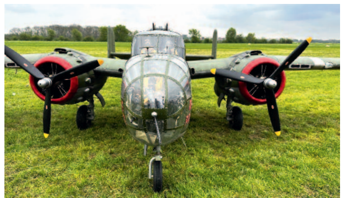
The large B-25, flown by Roland Sabatschus. The completely wooden model is powered by two Moki radial engines.
