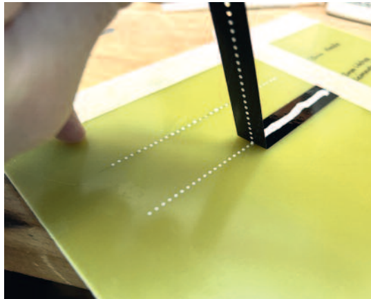
Step 3: After a short waiting time (approx. 60-90 seconds), slowly pull the rivet tape upwards.
