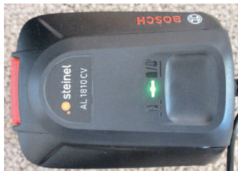
The Bosch Power For All battery on the charger. The flashing green LED indicates that charging is in progress. A continuous light indicates a full battery.
