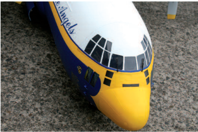
The add-on parts such as antennas, pitot tubes and windscreen wipers are not missing.
