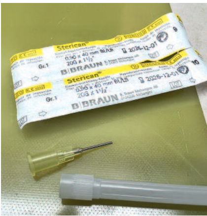
The basic equipment for the "syringe" method is a cannula from the pharmacy. Here a cannula with 0.9Å ~ 40 mm shortened to about 20 mm
