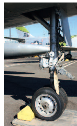
The undercarriage leg, which is hydraulically sprung with oil, moves backwards into the covered undercarriage shaft in the fuselage. The nose gear has two high-pressure tyres.
