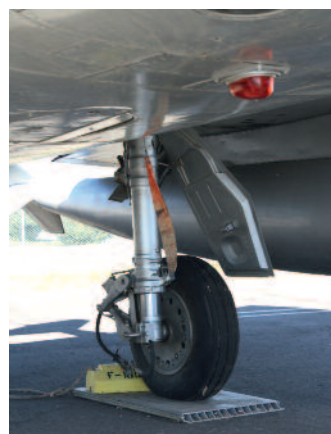
Like the nose gear, the main gear is hydraulically sprung against shocks during landing. However, the undercarriage leg has only one high-pressure wheel.
