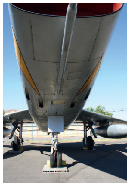
The undercarriage leg, which is hydraulically sprung with oil, moves backwards into the covered undercarriage shaft in the fuselage. The nose gear has two high-pressure tyres.
