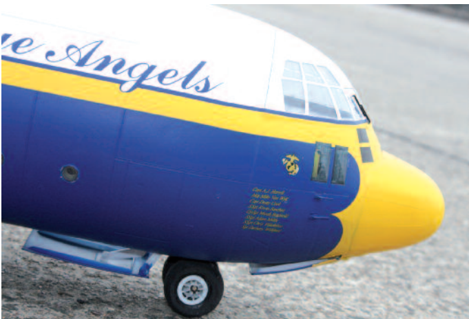
The plastic rims of the nose gear with twin tires could not withstand the stresses of rolling and had to be replaced with aluminum rims.
