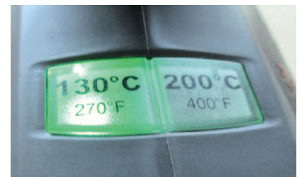
The gun is switched on by pressing one of the two temperature switches for a longer time. The illuminated switch flashes until the selected temperature is reached. After about two minutes, the light is on continuously and the gun is ready to start.
