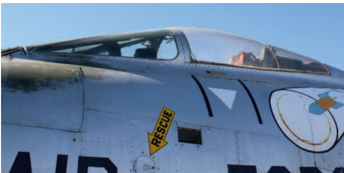
The teardrop-shaped cockpit canopy consists of one piece and can be opened and closed in normal operation by means of an electromechanical drive with an angle of 22°. In case of danger, the canopy is blown off the fuselage by an explosive charge, so that the pilot can eject safely with the ejection seat.
