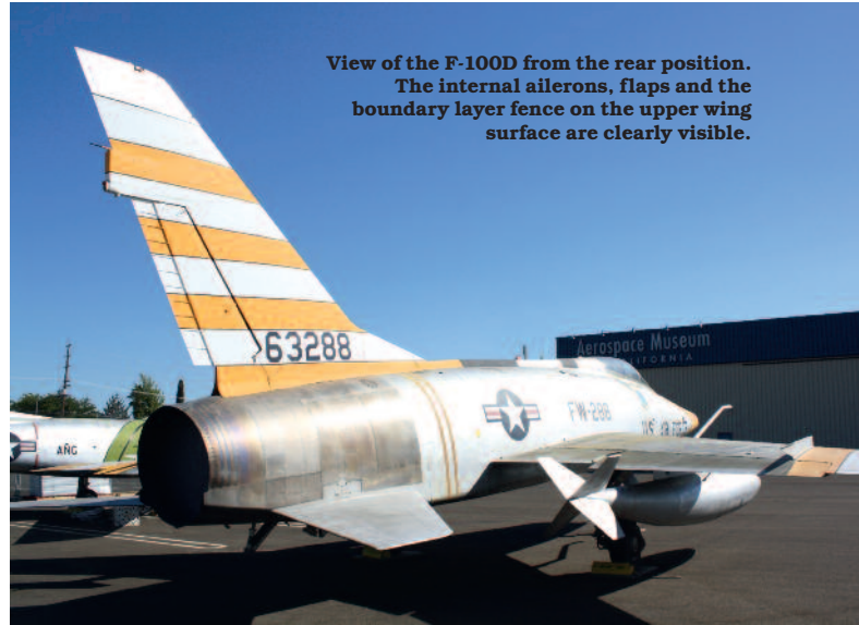
The wing of the F-100D has a sweep of 45° and a seven percent thickness ratio at the thickest point and a 3.5% ratio at the weakest point. Compared to the previous variants, the D-pattern has leading edge slats.
