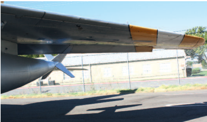
The aileron is located in the inner part of the wing for stability reasons. Wind tunnel tests have shown that an external aileron causes the relatively thin wing to flutter and oscillate in flight.
