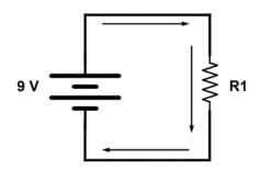
Resistance is the measure of the property of a material to oppose current flow. It's measured in ohms, symbolized by the Greek letter  $\Omega$ . The resistor is the component that uses its internal resistance to restrict current flow. This is the schematic symbol, and next to it, a normal resistor:
