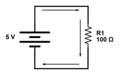
Here, we have one 5-volt voltage source in series with one resistor R1 with a resistance of 100  $\Omega$ . Because we have only one resistor, the total voltage across it will be equal to the voltage of the source, 5 V. We can now apply Ohm's law to find the current in the circuit:
