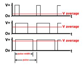
We can see in the first part of the graphic that we are mostly keeping the pin LOW, to 0 V, and thus the average voltage output is quite low. In the middle of the graphic, we are roughly keeping the pin HIGH and LOW for an equal amount of time, and the resulting voltage is half. In the last part, we see that the time the pin is HIGH is called Pulse Width. The total time between the beginning of each pulse is called the period of the PWM signal.
