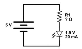
Due to the 1.9-volt drop across the LED, we only have 3.1 V across the resistor. Now we can apply Ohm's law to find the resistance:
