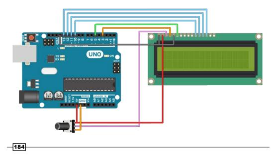
Follow these steps to connect an LCD to the Arduino:
