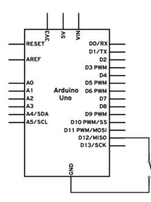
Here is a simple way of wiring the button:
