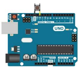
For most buttons with standard through-hole terminals, we can directly input the pins into the terminals on the Arduino.
