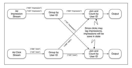
Figure 4.13 Handling ad impression and ad click streams that use stream state
