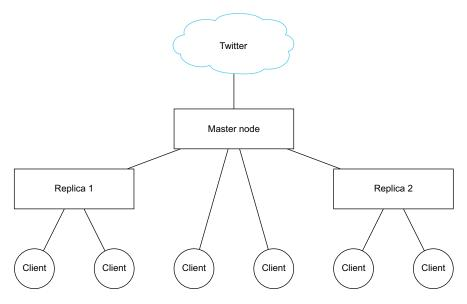
Figure 2.5 Scaling out using replica nodes
