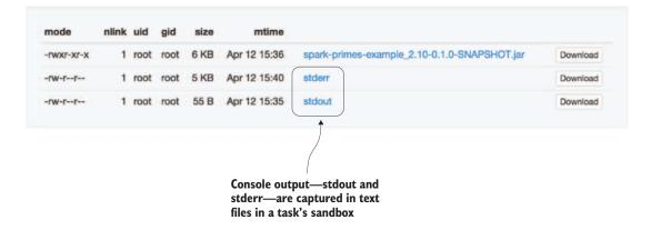
Figure 2.6 Files within a Mesos sandbox for a single Spark task
