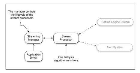
Figure 4.5 Turbine engine monitoring on our common architecture
