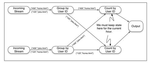
Figure 4.11 Simple example of counting page views per user over an hour
