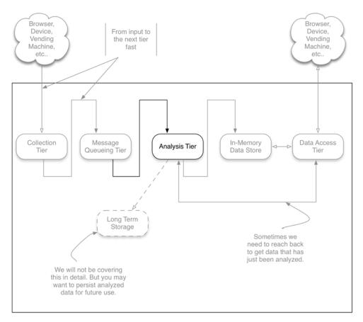
Figure 4.1 The streaming data architecture with the analysis tier in focus
