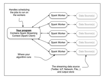
Figure 4.7 Spark Streaming high-level architecture
