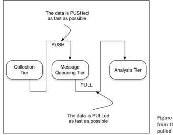
Figure 4.2 Data being pushed from the collection tier and pulled from the analysis tier
