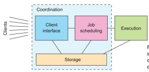
Figure 12.2 Intermediate component separation with the Coordination component being broken up in three distinct responsibilities.
