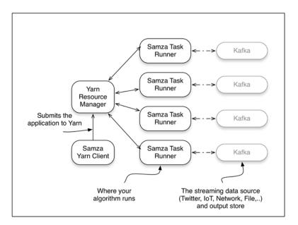
Figure 4.9 High-level Apache Samza architecture
