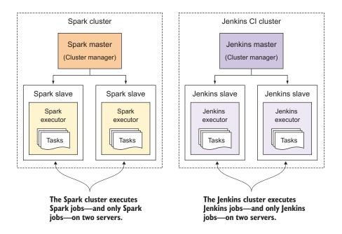
Figure 2.2 Visualizing two statically partitioned, or siloed, clusters
